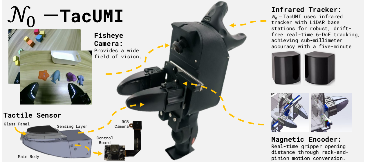
Figure 2 Overview of \mathcal{N}_0 -TacUMI. A single handheld unit records complementary streams: a fisheye camera captures the wide-angle wrist view, two camera-based tactile sensors capture contact-rich deformation at the fingertips, an infrared tracker with base stations provides a low-drift six-degree-of-freedom pose, and a magnetic encoder measures the gripper aperture through a rack-and-pinion transmission. The inset shows the layered structure of a tactile sensor, comprising a glass panel, an elastic sensing layer, the main body with an embedded RGB camera, and a controller board.
